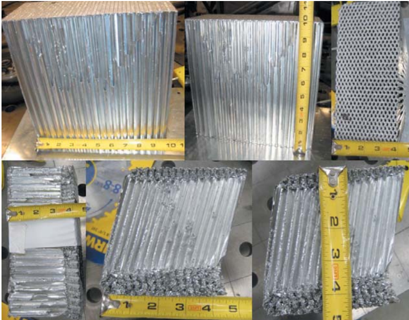
Figure 10: Sample 2 Impact Attenuator Before and After Testing.
